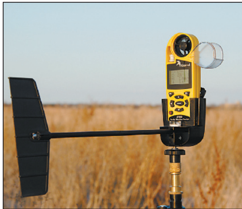
An optional base allows the weather station to accurately track wind direction or act as a data-log for automated collection of weather information. (WP photos by Michael Raine)
